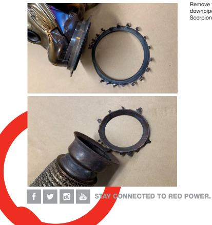
Remove the original gaskets from the original downpipe as they are required when fitting the Scorpion downpipe.
